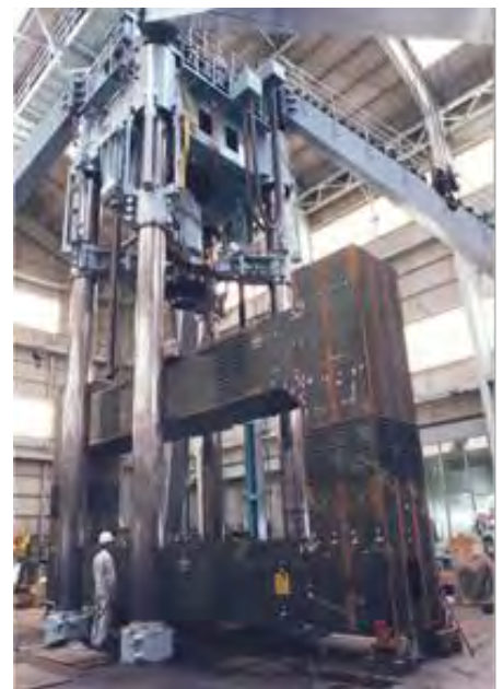
Photo 2. 4MN fatigue testing machine
