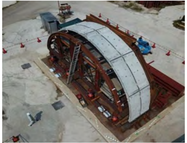
Photo 7. 2-ring assembled precast lining
